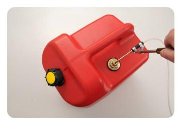
Cable tie fuel line and fuel pump wiring as required, <u>keep the fuel line a safe distance</u> <u>from the hot exhaust pipe.</u>
