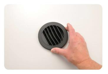
Attach ducting to the back of the outlet nut. Fasten with  $\emptyset$  60-80 mm jubilee clip using a 8mm hex socket. Pictured is 75 mm ducting.
