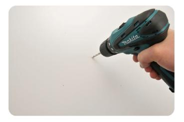
Drill  $\emptyset$  6 mm hole for mounting pump saddle. Assemble parts.
