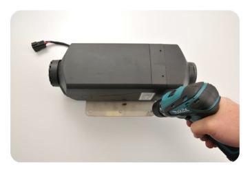
**Optional insulated floor mounting plate**. Connect fuel line, air intake and exhaust as 4.1-4.9. <u>Note the fuel pump cable does not</u> go through the mounting plate. If required drill a Ø 32 mm hole.
