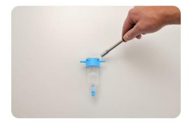
Connect fuel line to fuel filter. Butt fuel line to fuel filter spigot ends when adding rubber joiner to reduce air in the system. Use a 7 mm socket. <u>Do not over tighten</u>.
