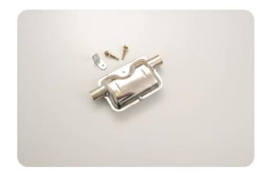
Fasten mounting bracket to heater as pictured using an 8 mm socket. HeaterX silencers are an 'S' design rather than straight through. This helps to capture hot exhaust carbon within the silencer and provides beater acoustic performance.
