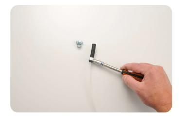
**7.5** Assemble fuel line to fuel pump as pictured. Butt fuel line to fuel pump spigot ends when adding rubber joiner to reduce air in the system. Use a 7 mm socket. Do not over tighten.
