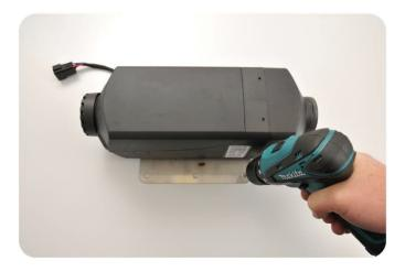
Fasten mounting plate to floor using own fasteners. Where possible we recommend using a bolt, nut, flat washer, and spring washer for a secure fit. Fastens not supplied in kit due to installation variances.
