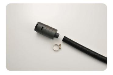
Fasten air intake hose to air intake silencer as pictured. Use 7 mm socket. <u>Do not over tighten</u>.
