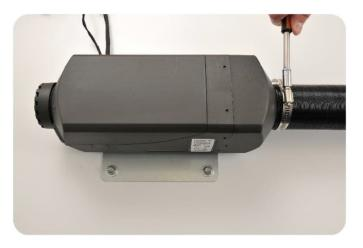
Drill  $\emptyset$  3 mm pilot hole for the centre of the hot air outlet duct.
