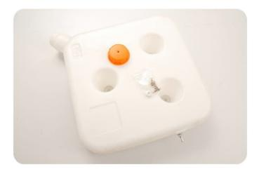
Mount the tank with filler cap at top and supply spigot at bottom. <u>Supplied tank is not</u> <u>designed for outdoor use. UV damage will</u> <u>cause it to become brittle over time</u>.
