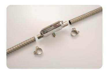
Make a small cut into ID  $\emptyset$  24 mm exhaust hose as pictured. This will allow a correct compression when clamped.
