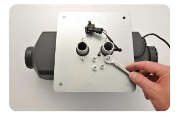
Use 1 x rubber fuel connector, 1 x 9-11 mm jubilee clip and fuel line. Join as pictured using a 7 mm socket. <u>Do not over tighten</u>.
