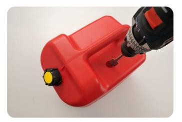
**7.18** Lower standpipe as pictured. Measure length of standpipe required and cut to suit. Check the standpipe straw is open and clear after cutting. Cut the standpipe 10 mm from the bottom of the tank to reduce contaminants from entering the fuel system.
