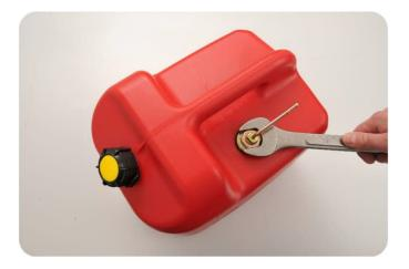
**7.21** Use 1 x rubber fuel connector, 1 x 9-11 mm jubilee clip and fuel line. Join using a 7 mm socket. <u>Do not over tighten</u>.
